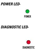
This indicator illuminates during the power-on self test, then should turn off. If it remains illuminated, this indicates that the self-test has detected an unexpected event, such as a corrupted firmware update via TFTP or a memory boot failure. If the DIAGNOSTIC LED remains illuminated, try resetting the CM16a by cycling power off and
